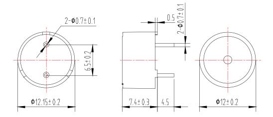
\*Unit: mm; Tolerance: ±0.5mm Except Specified \*Housing Material: Black PBT
