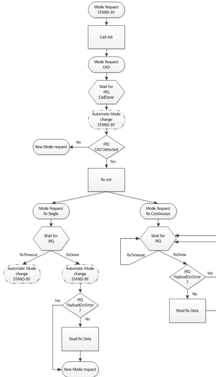
Figure 10. LoRa™ CAD flow
