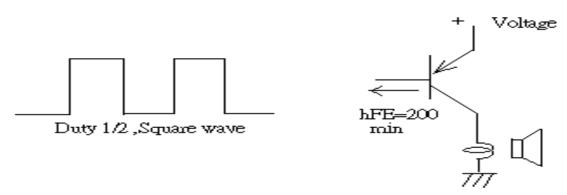
The base current Ib should high enough so that it saturates the collector current of the transistor with the CB load.
